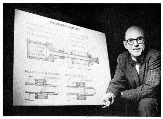
MANGANIN GAGE, held in fingers of Edward O. Williams (8112), was used in development work for which he received the annual Vigness Award as the author of the outstanding paper on the subject of shock and vibration. Laboratory tests on the illustrated helium-driven pneumatic hammer have proved the ability of the Manganin gage to measure up to 104 kilobars of pressure while installed inside a material sample.
